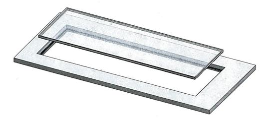
3. Insert all for thermal breaks and insert them into the front frame.
